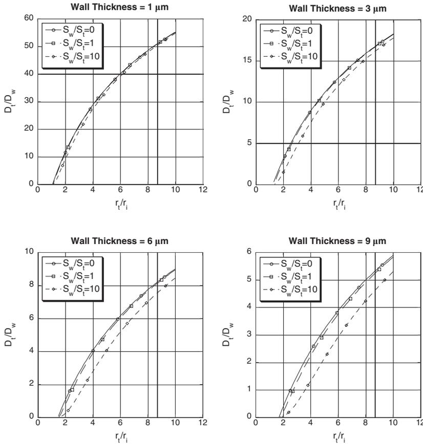
**Figure 2** Diffusion enhancement factors as a function of the linear size of the interstitial basin supplied by the arteriole for various wall thicknesses and the ratio of consumption rates in the wall and in the interstitium. The vertical lines indicate the values as measured in the experiment.
