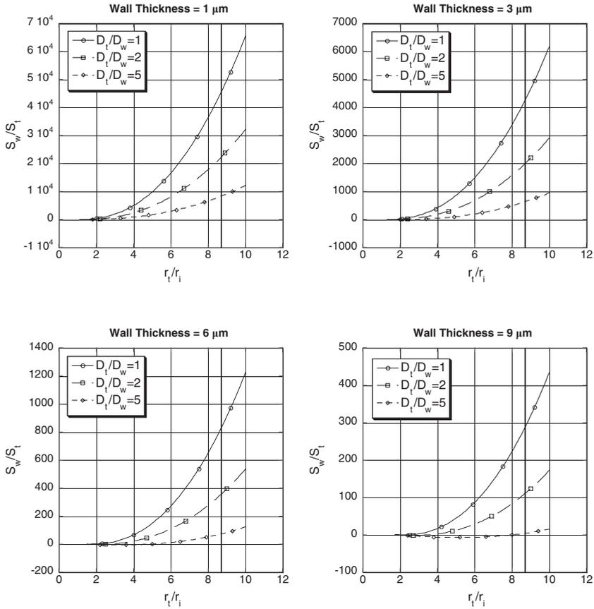
**Figure 3** The ratio of consumption rates in the wall and in the interstitium as a function of the linear size of the interstitial basin supplied by the arteriole for various wall thicknesses and diffusion enhancement factors. The vertical lines indicate the values as measured in the experiment. Note that for a wall thickness of  $9\ \mu\text{m}$  and a diffusion enhancement of 5, the resulting consumption ratios fall outside the physical range and take on negative values.
