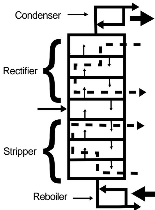
Figure 2: Conventional column retrofitted with serial heat exchangers.
