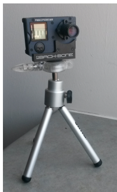
Figure 1.1: RibCage Air Modified GoPro Hero 4 Black camera with a 25mm f/2.0 14d HFOV 3MP lens on its tripod.
